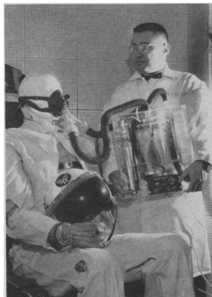
SPACE TEST —Miniaturized instruments developed by the Boeing Airplane Company are shown on a life-size model. The 15-pound metabolism measuring instrument held by Dr. Irving Streimer was trimmed down from the normal 100-pound device.
