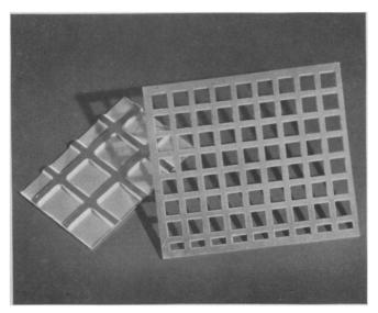
New methods of metalworking do not come along often enough to be ignored. Here are two examples of what we call "photo-milling." The one on the right could, of course, have been done on a punch press if die cost had been justifiable. No die was used, nor were the openings cut individually. The one on the left looks like a milling machine job, for sure. It isn't.
