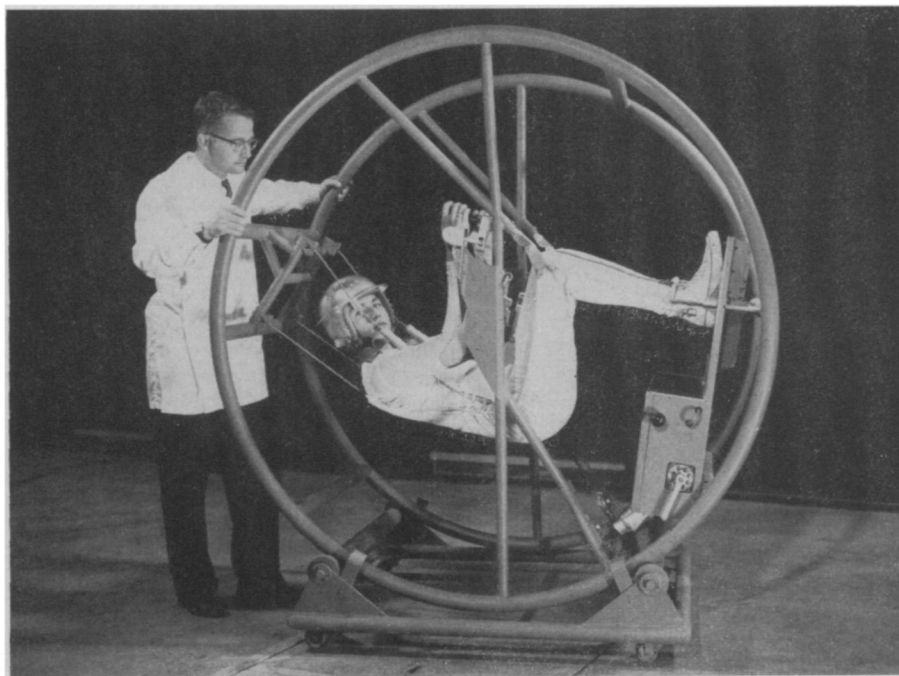
SEAT-SUIT —Suspended in boost or blastoff position, Gary Grabam, Boeing Airplane Company engineer, models the "hammock-seat" restraint system he developed. The device is made of nylon net with steel cables sewn into it seems. Engineer Peter Downey operates the cabin simulator.
