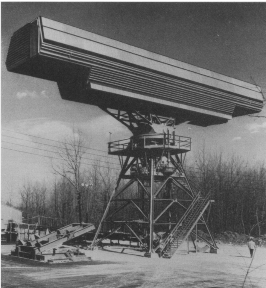
SUPER SENTRY —The rotating 50-ton "boxcar shaped" radar antenna will warn against air-attack as part of the nation's defense network. It is 104 feet long and was developed for the U. S. Air Force by Raytheon Company. The antenna array is called a considerable advance in radar. It can detect invaders hundreds of miles away.
