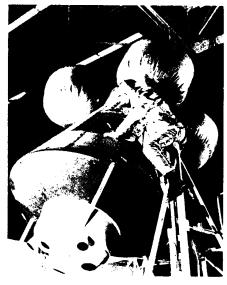
SPACE CAPSULE—A pilot is getting ready to climb into a model of the manned satellite being built for the National Aeronautics and Space Administration by McDonnell Aircraft Corporation. The retro-rockets (lower left) and the flotation bags give the capsule bouyancy and stability in water.
