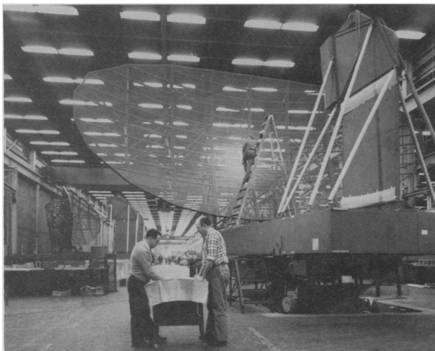
LAND-BASED RADAR —The first land-based radar antenna to combine height, distance and direction finding capability in a single unit is shown in final assembly at the General Electric ordnance department, Pittsfield, Mass. The seven-ton antenna is part of the SAGE continental air defense system.
