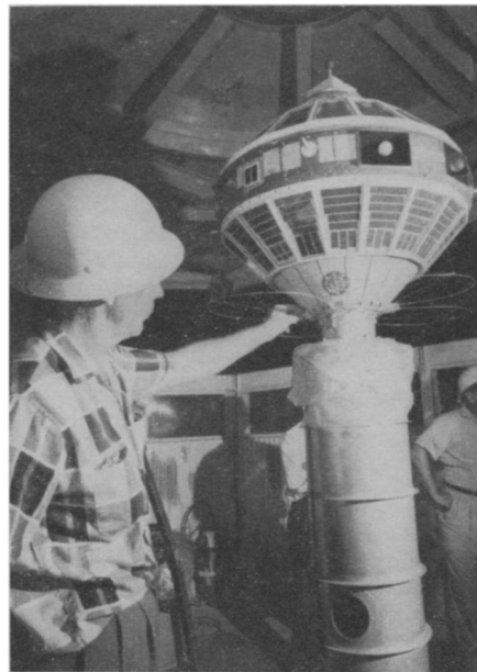
EXPLORER VII —One of the scientists inspects the satellite on the fourth stage of rocket prior to the launching of the Juno II rocket carrying Explorer VII, with a 91.5-pound satellite into orbit. The launching was under the direction of the National Aeronautics and Space Administration, at Cape Canaveral, Fla. (See p. 301.)
