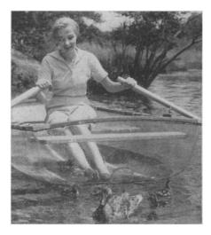
horsepower motor. It is eight feet long and weighs less than 50 pounds. Hull transparency, illustrated in the photograph, permits easy study of marine life or quick selection of sites for fishing and skin-diving.
