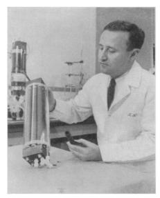
NEW POWER PACKAGE—The device being held by Dr. Karl Kordesch of the National Carbon Company is a fuel cell capable of generating electricity when hydrogen and oxygen gases are fed into its special nine hollow, porous carbon electrodes. In operation, the fuel cell is filled with potassium hydroxide. It generates electricity as long as hydrogen and oxygen are fed in, and requires no recharging.
