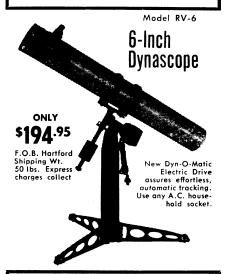
Finest American-made 6-inch reflector in its price rangel Save \$100 or more, yet get all these fine features: f/8 6-inch mirror accurate to  $\frac{1}{8}$  wave • electric drive • 3 matched eyepieces (75X, 150X, 343X) • 6x30 Achromatic finderscope • Heavy-duty mount with setting circles • Rack & Pinion eyepiece holder • Rotating tube • Sturdy lightweight tripod.
