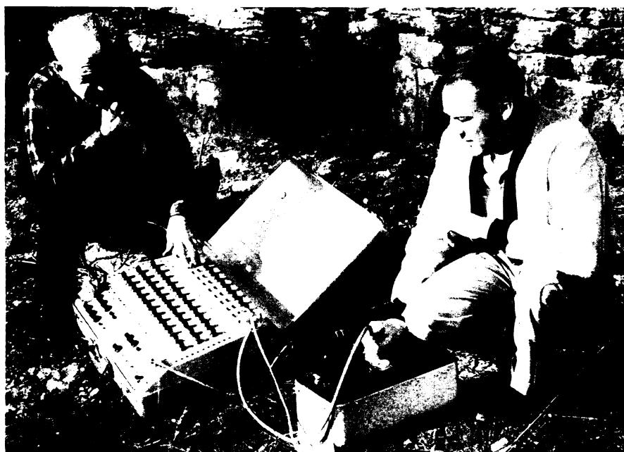
PORTABLE SEISMOGRAPH SYSTEM —For surveying shallow rock formations, Sinclair Research Laboratories, Inc., Tulsa, Okla., developed this miniaturized seismograph system that works to a depth of 2,000 feet. The equipment can be carried by two men. Al C. Reid (left) is making instrument settings while Lester J. Smith (right) stands by to operate the data recording camera.
