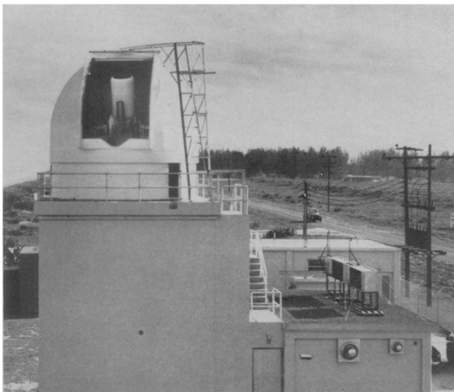
INFRARED SCANNER —Infrared spectrometric studies of missiles fired from Cape Canaveral, Fla., are being made with an infrared rapid scan instrument. It was built by Perkin-Elmer Corp., Norwalk, Conn., and is located at Melbourne, Fla. The infrared measurement program, conducted under an Air Force contract, includes the nature and rates at which time reactions occur during powered flight. (See story opposite page.)
