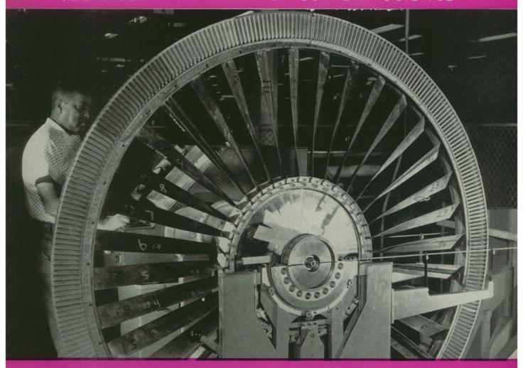
**VTOL Lift Fan Rotor**
