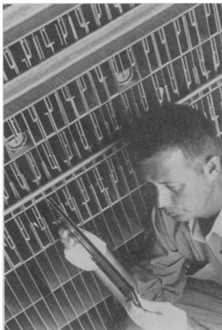
NUCLEAR HONEYCOMB — This nuclear assembly holds more than 4,000 uranium-aluminum foils as fuel. Chain reactions in the assembly will provide scientists at General Dynamics Corporation, San Diego, Calif., with data for development of the maritime gas-cooled reactor.
