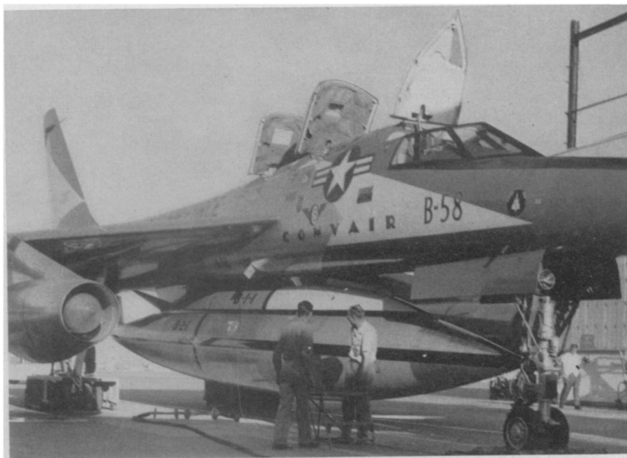
DROPPABLE POD —A two-part droppable pod provides extra speed and mileage to the Air Force B-58 bomber. The fuel-carrying lower part of the pod can be dropped when fuel is used. The upper part, containing a nuclear bomb, would be carried on to target in actual combat. The pod is in production at Convair Division of General Dynamics Corporation, Fort Worth, Tex.
