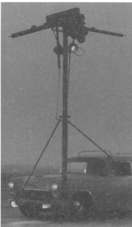
HIGHWAY GETS CHECK-UP— The antenna on top of the automobile is a photo-recording device for inspecting highway surfaces.
