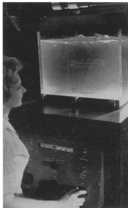
3-D PLOTTER —A three-dimensional plotting device has been developed by Chrysler Corporation Missile Division engineers to record paths of rockets, satellites and aircraft.
