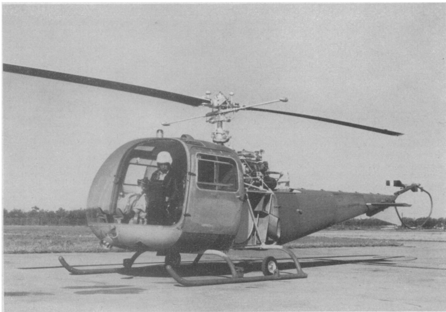
FIRST OF NEW GENERATION—The Navy HUL-1M utility helicopter is called the first of a new generation of turbine-powered light helicopters. The HUL-1M is the first aircraft to be powered by an Allison T-63 250 shaft horsepower turbine engine. It is now being tested at Bell Helicopter Company's plant at Fort Worth, Tex.
