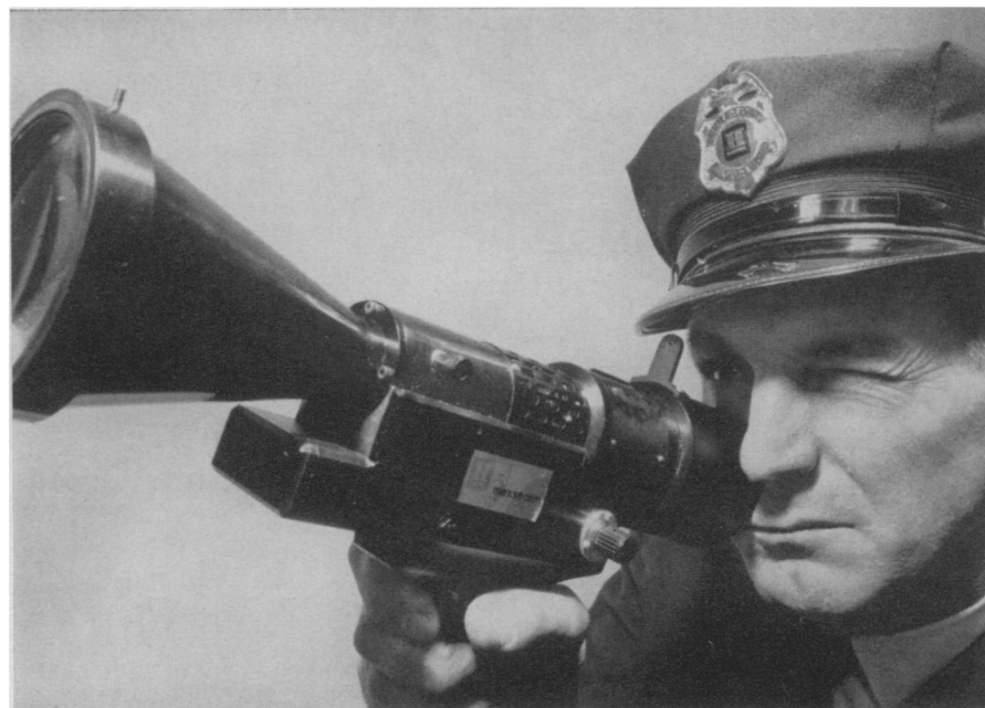
TALK BY RAY GUN —Words spoken into a "ray gun" are electronically converted to infrared beams and transmitted to a similar receiver several miles away that converts the message back to sound. The system was developed by Minneapolis-Honeywell Regulator Co. for use in military, police and civil defense operations.
