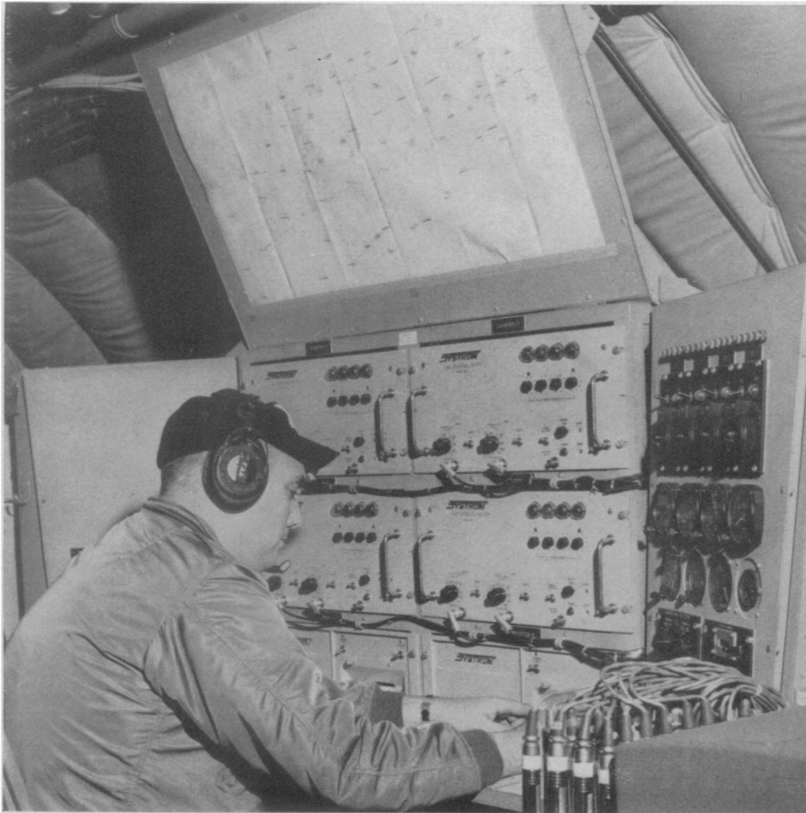
CHECKING FLIGHT AIDS —Navigational aids are checked for errors with SAFI (Semi Automatic Flight Inspection), a complex electronic system.
