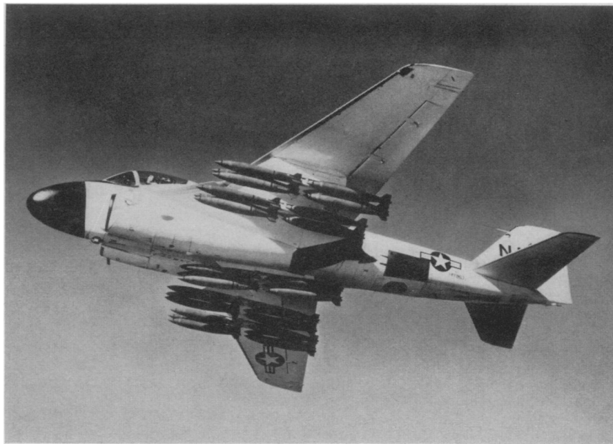
LOADED DOWN —The U. S. Navy's light attack aircraft, the Grumman A2F-1 Intruder, carries 30 five-hundred-pound bombs in clusters of three. The all weather plane was designed for troop support.
