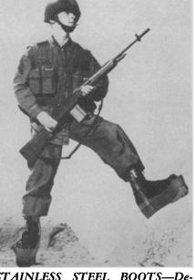
STAINLESS STEEL BOOTS—Developed by the Naval Medical Field Research Laboratory at Camp Lejeune, N. C., the new boots have a six-inch stainless steel "sole" with a "blast deflection" contour wedge to scatter fragments of exploding land mines from the wearer. They are expected to be issued to foot soldiers in 1962.
