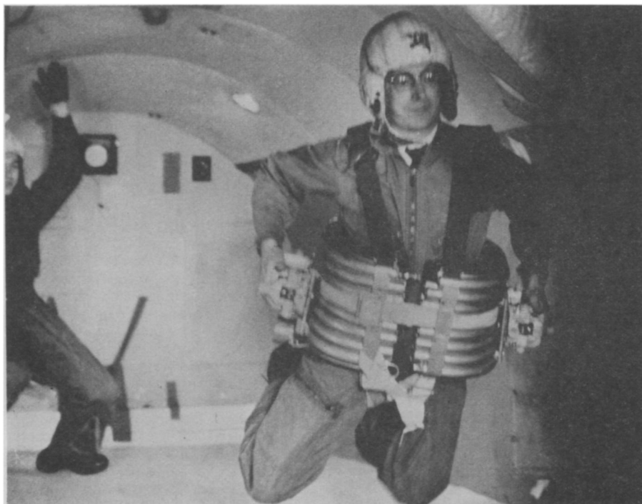
ZERO GRAVITY BELT —Scientist Ralph E. Flexman tests under zero gravity conditions a belt that will enable men to leave orbiting space vehicles to perform inspection, repair and assembly tasks in space. The belt is being developed by Textron's Bell Aerosystems Company, Buffalo, N. Y.
