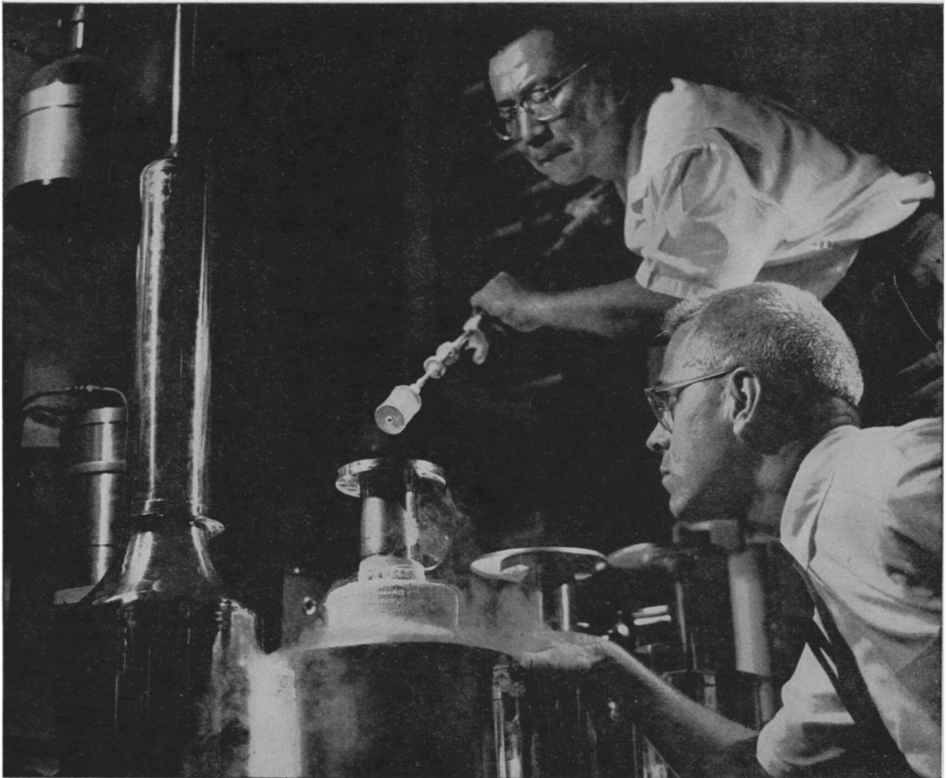
The Making of a Magnet. Bell scientists test new superconducting electromagnet, the small cylindrical object being removed from helium bath at minus 450 degrees F. An early experimental design produced a field strength over 65,000 gauss.
