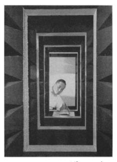
NO ECHO HERE—The windowlike openings, framed in foam, lead through an echo-free chamber developed by Republic Aviation Corporation's research center, Farmingdale, N.Y. In the chamber radio waves can act as they would in empty space. Model being inserted is undergoing radar measurement tests.
