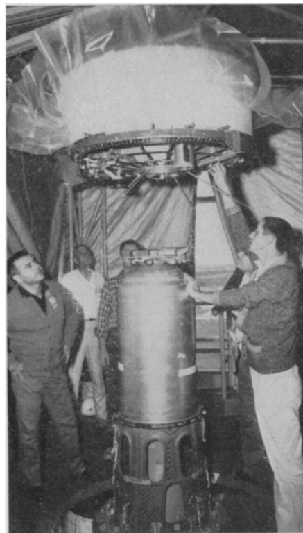
FIT FOR TIROS—The 284-pound Tiros IV is being fitted on top of the Thor-Delta booster.
