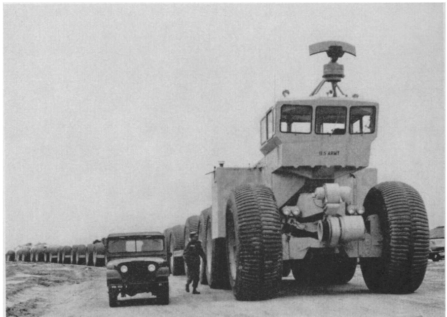
TRACKLESS TRAIN —A 572-foot overland train, designed to move supplies over desert or arctic terrain, has been completed for the U.S. Army by R. G. LeTourneau, Inc., Longview, Tex. Each wheel of the train is powered with its own drive motor and gear. Gas turbine engines and generator sets in the two rear cars supply electricity.
