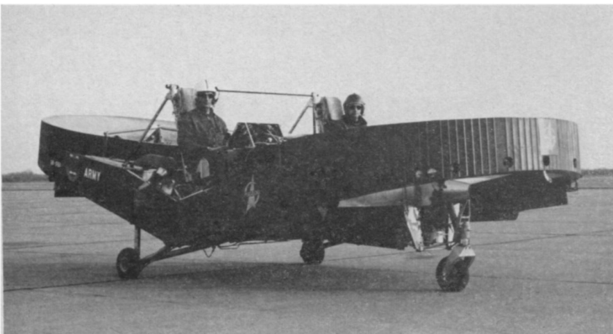
AIRGEEP II —A new, improved "aerial jeep" is powered by two turbines. Made under contract to the U.S. Army, the vehicle, developed by Piasecki Aircraft Corporation, Philadelphia, is currently undergoing testing.
