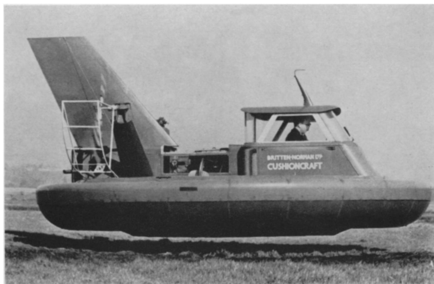
CUSHIONCRAFT PROTOTYPE —This version of a British hovercraft, powered by a sports car engine, travels 15 inches above land or water. A compressor around its circumference gives it lift through single jet nozzles.
