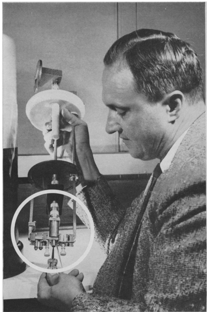
Bell Laboratories' Michael Chroney adjusts waveguide assembly (in circle) housing the diode. After adjustment the entire parametric amplifier will be immersed in liquid nitrogen in dewar at left. The new amplifier operates at 4170 megacycles (center of band) and provides an almost flat gain of 38 db over a 50-megacycle band with a noise figure of approximately 0.6 db.
