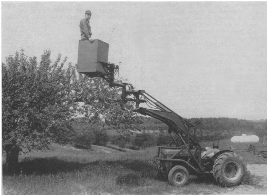
SPACE BASKET —To make pruning more efficient, a "space basket" is attached to the front-end loader of a tractor-mounted hydraulic-powered pruning and picking machine. The unit can move up and down and each arm section can move through an arc of 330 degrees horizontally.
