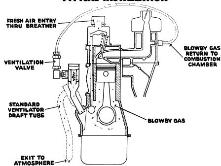
BLOW-BY DEVICE—A typical blow-by device for a six-cylinder engine, used to control air pollution. An adapter (left) is placed on the crankcase to draw hot vapors from the car's system. These are returned (upper right) to the combustion chamber where they are further reduced after re-entering the system.
