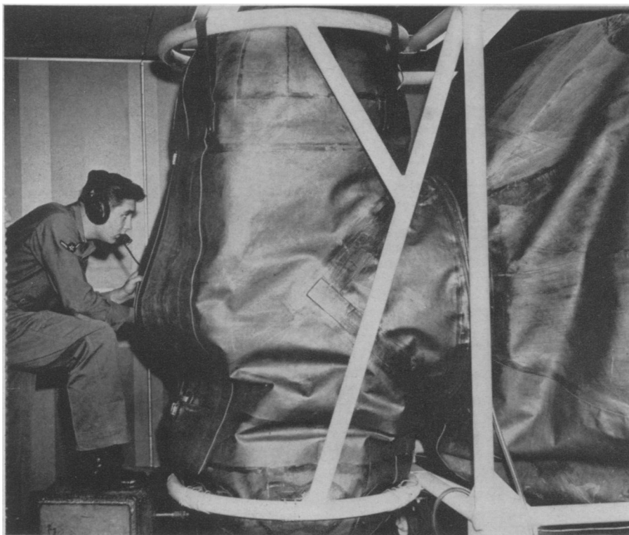
VOLUNTEERS ZIPPED IN —An airman zips shut the space cell in which Air Force volunteers are sealed to determine their reactions to various atmospheric pressures and compositions. The cell was built by Goodyear Aircraft Corporation at Wright-Patterson Air Force Base in Dayton, Ohio, for research on the best simulated atmosphere for long space flights.
