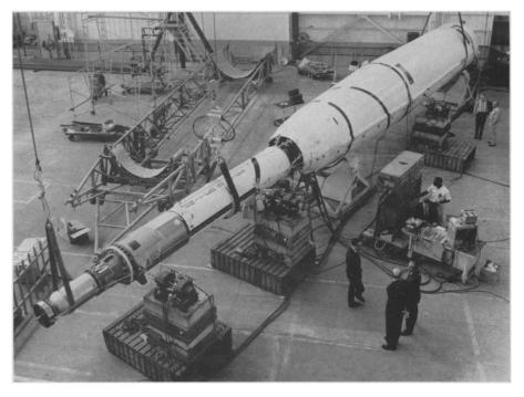
VIBRATION TEST—A fully assembled Douglas Delta space vehicle, similar to the type that will launch the National Aeronautics and Space Administration's Relay communications satellite, is put through a vibration test at the Santa Monica, Calif., facility of the Douglas Missile and Space Systems Division. The 80-foot-long, 8,428-pound vehicle was suspended from cables for the test, which determined vehicle control stability and vehicle body bending modes.
