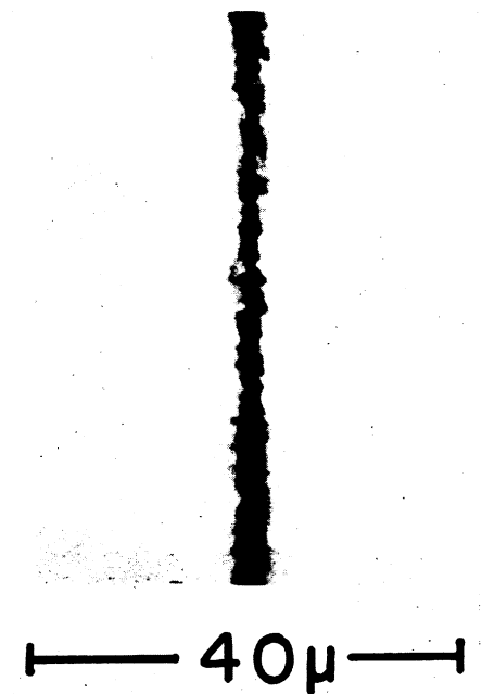
COSMIC RAY PATH —A microscopic photo shows the trail left by a cosmic ray through the interior of one of the silver chloride crystals developed by Dr. Lawrence M. Slifkin of the University of North Carolina department of physics. The trail has been made visible by a special process. The actual width of the trail shown is no more than one-tenthousandth of an inch.
