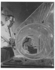
DRY BOX allows scientists at The Goodyear Tire & Rubber Company, Akron, Ohio, to experiment with chemicals requiring an absolutely dry and inert atmosphere.
