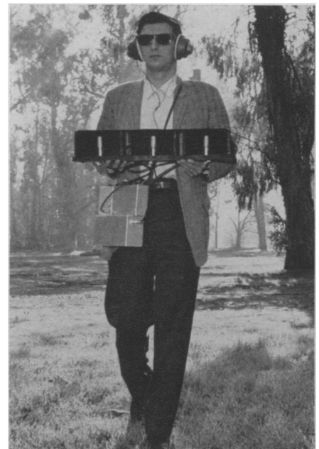
BAT RADAR DEVICE —Alvin E. Brown, research scientist of Lockheed Missiles and Space Company, finds his way through a wooded area with a bat radar device developed to help the blind.
