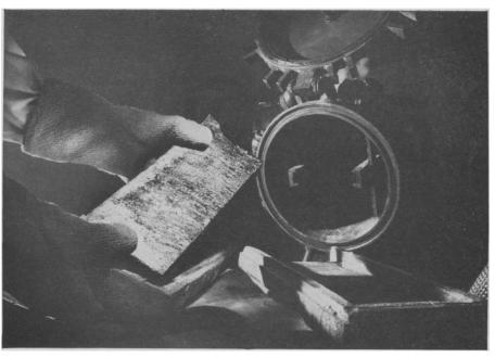
Ingot of high-purity nickel alloy is removed from controlled atmosphere melting furnace. Alloy is virtually free of impurities which inhibit electron emission. The new alloying technique and the methods for making cathodes and evaluating their electron-emitting properties were developed by K. M. Olsen and H. E. Kern.
