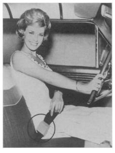
driving safety by making it impossible to start a car until the seat belt is fastened securely by the driver. When the seat belt is tightened, the pressure trips a safety mechanism unlocking the car's starter. Easily installed, it will not interfere with the operation of the car.
