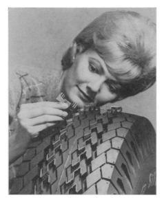
which put vertical ridges inside the grooves of truck tires. Besides making the tires more rugged, the ridges keep out small stones and increase wear by reducing the squirming action of tread elements as they contact the road. The new tread pattern and a new wear-resistant rubber produce a tire that has averaged 32% more mileage than other similarly priced tires.
