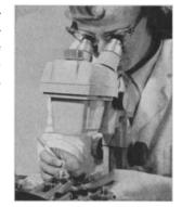
erations without damage to delicate parts. A turning of the zoom dial gives continuously variable magnification without altering working distance.
