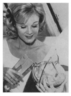
tool can be used to join plastics, fabric, rubber and other materials, as well as metal. Taking only a few seconds to operate, the rivet is set from one side merely by placing the stem in the tool and inserting the rivet into the hole of the work and squeezing the handle. The joint does not loosen by vibration or service. An assortment of rivets and back plates is included in the riveting kit.
