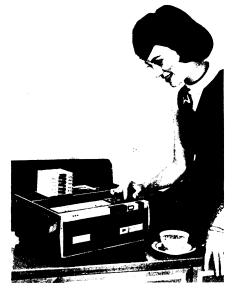
AUTOMATIC TAPE RECORDER-PLAYER, shown in photograph, provided with an automatic tape-changer produces 15 hours of continuous stereophonic music. Simple to operate, the recorder-playback will play taped cartridges automatically, performing all operating functions, including threading of the tape, playing, rewinding and advancing to the next cartridge. Up to 20 tape cartridges can be played in succession without interruption.
