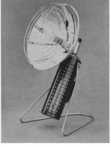
in the shown in photograph, ideal for outdoor as well as indoor use, produces instant direct-ray heat at the touch of a match and without electricity. A small cigar-shaped core which glows instantly generates infrared heat projected by a reflector to heat boats, trailers or cabins. Having no flame, the unit is windproof. The heater also can broil, heat frozen foods and dry hair, clothes or paint.
