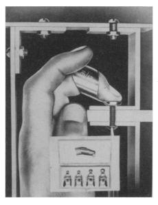
tiny nuts firmly on the fingertip simplifying work in snug, narrow and blind areas. The handy wrench that slips like a ring over the finger has a specially devised projection that fits over the nut and holds it securely while working. A set of four sizes are encased in a sturdy plastic storage box.
