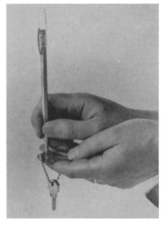
DIAMOND POINTED MARKER, shown in photograph, writes on rocks, tools, surgical instruments, machine parts, sports equipment, laboratory glass and other materials as readily as a pencil on paper. The marker, which consists of a diamond point set on the end of an aluminum stem, is no larger than a ball point pen and can be carried in a shirt pocket. It is also useful to homeowners for mark-
