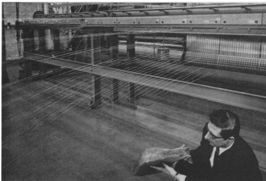
LOOM TO WEAVE STEEL —Stainless steel strands that are used to make Airmat material are shown being fed into the giant loom. An engineer inspects a sample of the finished product with the metallic threads stretched between the outer surfaces.
