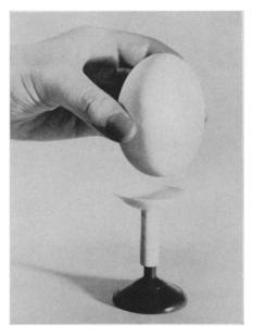
while being boiled, eliminating misshapen hard- or soft-boiled eggs. Before cooking, the larger end of the egg, which contains the air pocket, is pressed down into the piercer. A steel needle punches a tiny hole through the shell. This allows the air confined in the shell to escape as the egg is cooked and thus prevents the shell from breaking.
