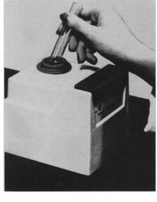
WORTEX-ACTION SHAKER, shown in photograph,  $4\frac{1}{2}x5\frac{3}{4}x5\frac{1}{2}$  inches in size, agitates individual test tubes, flasks and bottles up to 40mm in diameter in a one-handed operation. The user holds the sample against the oscillating neoprene cup while his palm depresses the broad switch plate. By varying the pressure and angle of the vessel, the degree and rate of mixing can be controlled.
