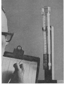
RAIN GAUGE, shown in photograph, is made of transparent plastic and enables farmers, ranchers, gardners and hobbyists to accurately measure local rainfall. Having a capacity of five inches of rain, the sturdy gauge comes with a rustproof bracket and can be easily installed on fence or post. Easyto-read graduations are shown in black at one-half-inch intervals.
